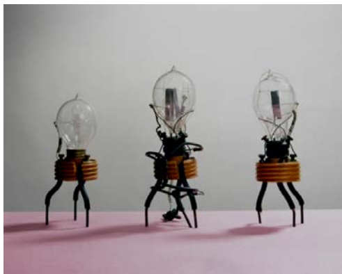
Fig. 4. Primele diode termionice inventate de Fleming, 1904 (sursa: https://collection.sciencemuseumgroup.org.uk/ ).
